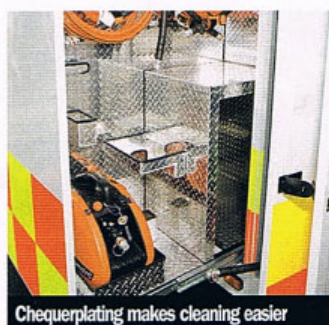
Chequerplating makes cleaning easier
