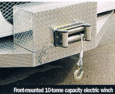
Front-mounted 10-tonne capacity electric winch
