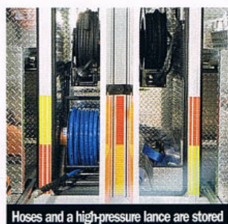
Hoses and a high-pressure lance are stored
